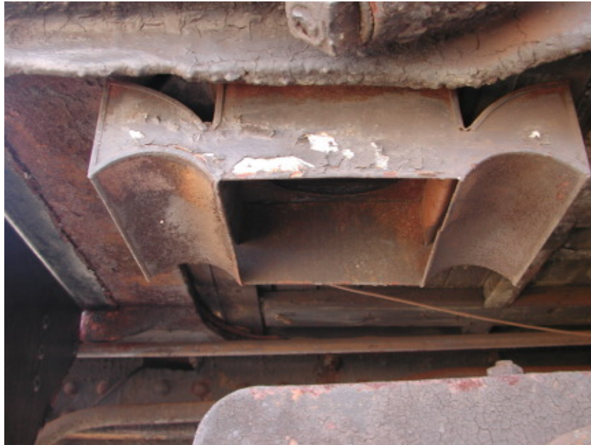
Cute little venturi for downdraft, unfortunately placed over truck frame.
